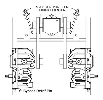
Each hydrostat has a bypass relief pin located at the rear of the hydrostatic unit. A bypass keeper is provided to allow the mower to be rolled around without engine running. To accomplish this, the bypass keeper springs must be positioned to depress the bypass relief pins. Remove bypass keeper springs prior to actual operation of the mower.
